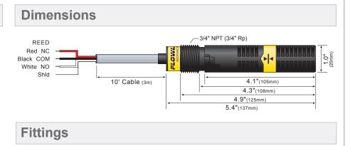
For optimum performance, install the level sensor using the below recommended or direct equivalent fittings.
